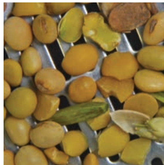
▲ Parts of soybean sample on the 1,8 mm slotted sieve (according to dispensation).
