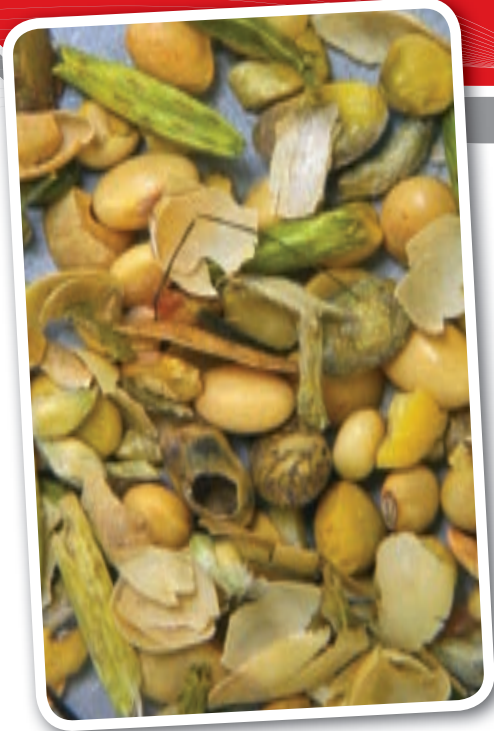
▲ Parts of soybean sample which passed through the 4,75 mm round hole sieve (prior to dispensation).
