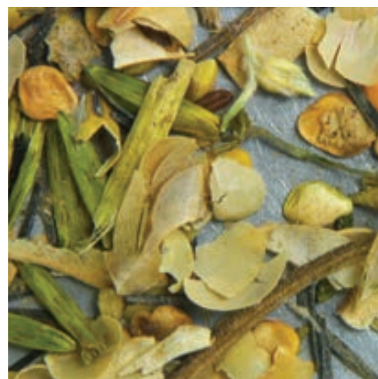
▲ Parts of soybean sample which passed through the 1,8 mm slotted sieve (according to dispensation).
